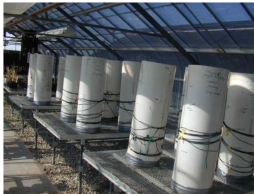
Bench-scale soil column tests
