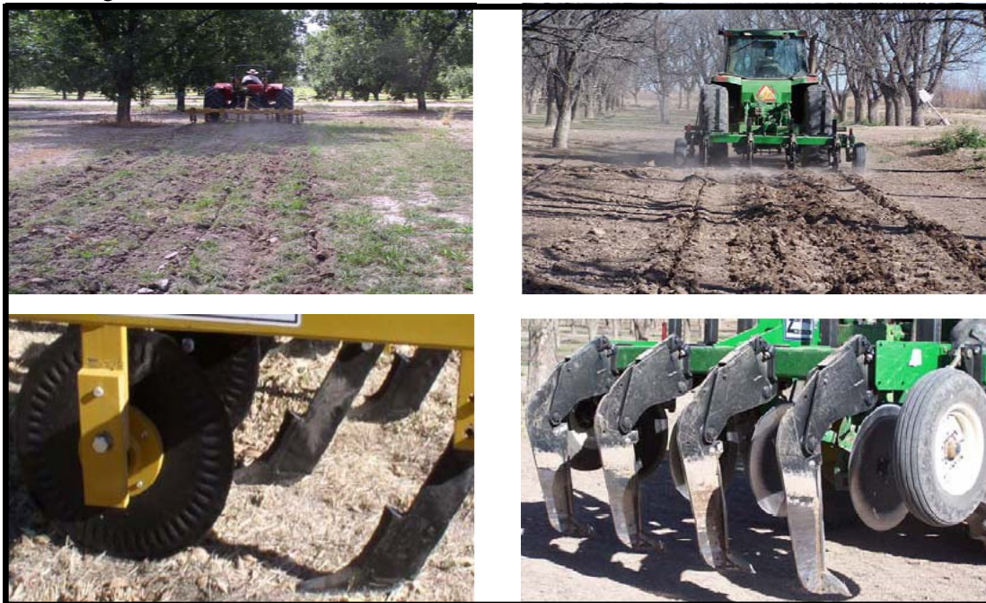
Soil management practices at a pecan orchard using the minimum-till surface chisel (left) and minimum-till subsoiler (right).
