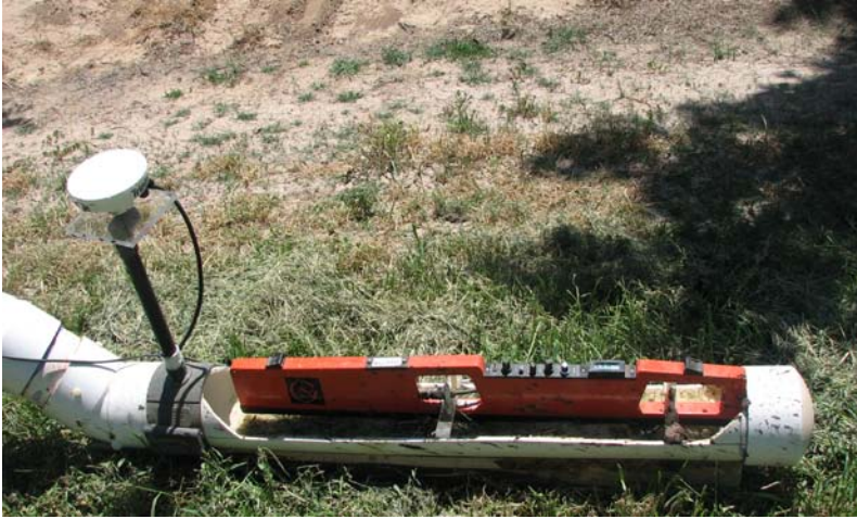
Electromagnetic induction meter fitted with GPS unit
