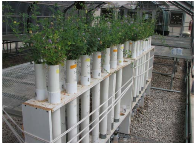
Greenhouse soil column study evaluated cooling tower reject water irrigation effects on alfalfa performance, soil salinity, and leachate chemistry.
