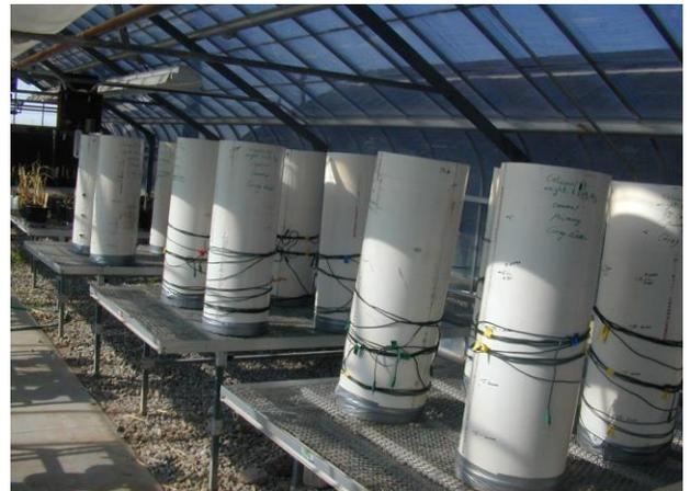
*Bench-scale soil column tests*
