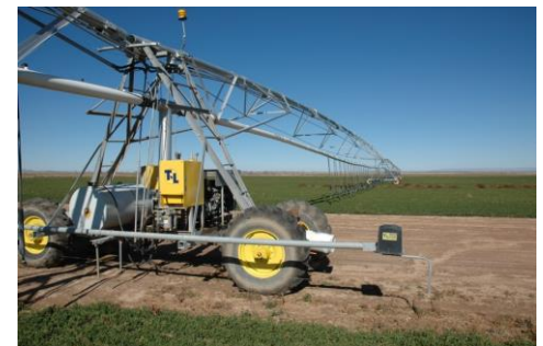
Low pressure linear sprinkler system
