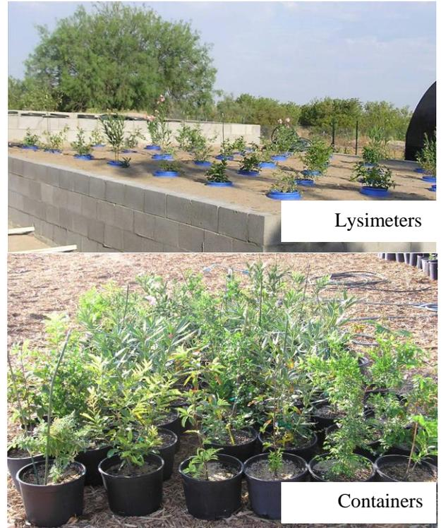
*Parallel experiments were conducted by growing the same species in lysimeters and containers. Their water use and crop coefficients were determined and compared.*
