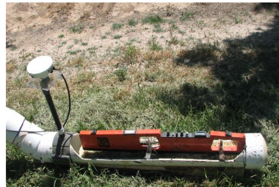
Electromagnetic induction meter fitted with GPS unit
